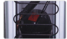
Hermetically sealed reciprocating Compressor
